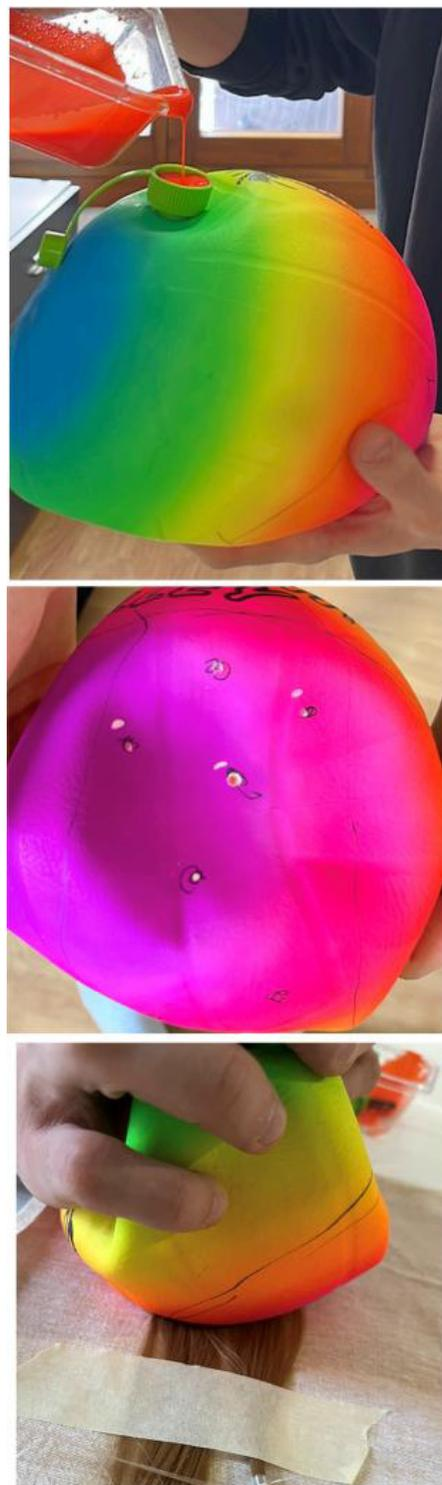
**Figure 7:** Experimental test performed simulating the occipital region using a PVC balloon. The balloon filled with red fluid (top) was then pierced (center) and, pressurized, brought into contact with hair and fabric.
