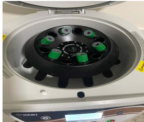
Figure 7: Poor balancing can cause excessive shaking, which in turn negatively impacts platelet activation. When the tubes are perfectly balanced, the centrifuge operates smoothly and efficiently, ensuring that the platelets are activated in a controlled and uniform manner. This is crucial for achieving a high-quality PRP.
