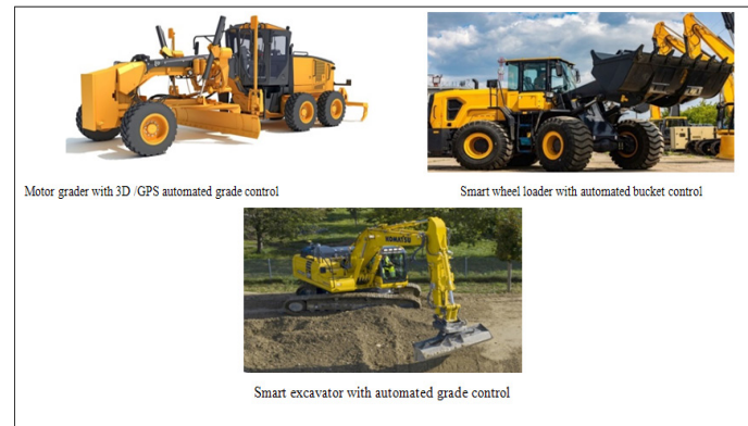
Figure 4: AI – Driven Smart Construction Equipment and 3D GPS AMG.
